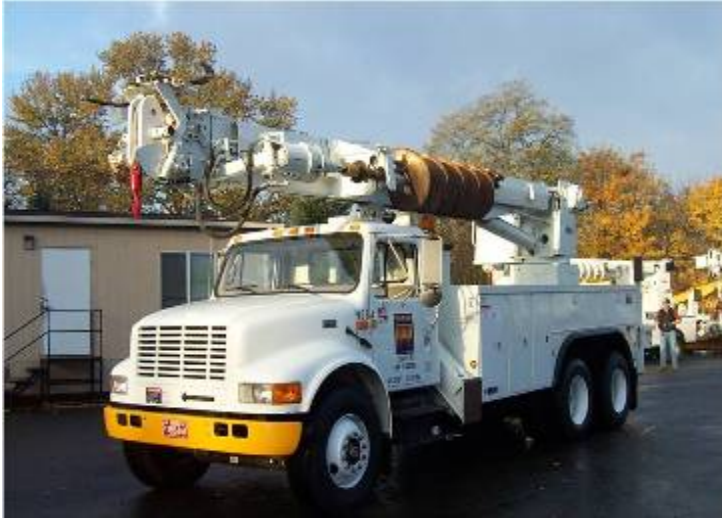
Photo of a digger derrick.
